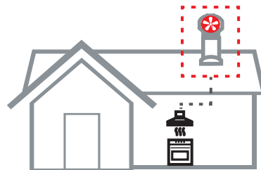
Kitchen cooker hood and a fan on the roof - silent kitchen
