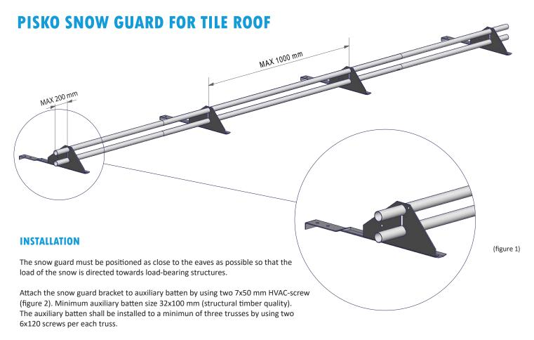
Slide the snow guard pipes through the round holes of the roof brackets and secure the pipes in place by pipe fixing screws through the pipes, next to the outmost brackets.
